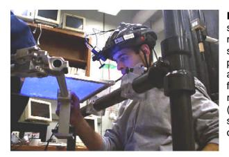
**Figure 2.1**. Experimental setup with the subject gripping the robotic manipulandum. A drape (not shown) surrounded the horizontal screen to prevent the subjects' vision of their own arms. A bite bar was used for head fixation, while a helmet-mounted camera recorded eye position. A LCD projector (outside the field of view, above the subject's head) projected visual stimuli onto the screen.
